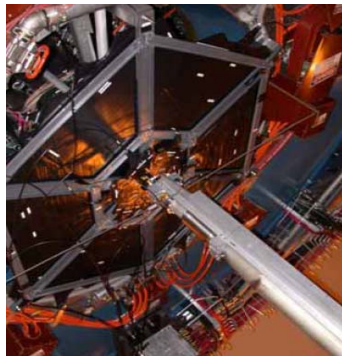
STAR Beam-Beam Counter Schematic Front View
